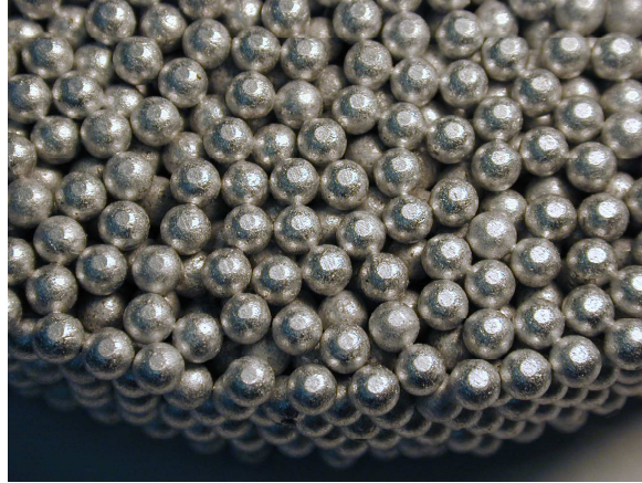
Fig. 1. – One of the samples in which the localization of ultrasonic waves was observed in the intermediate frequency regime. The aluminum beads are brazed together with weak elastic links to form a disordered solid network, in which the ultrasonic waves become trapped after strong multiple scattering from the pores.
