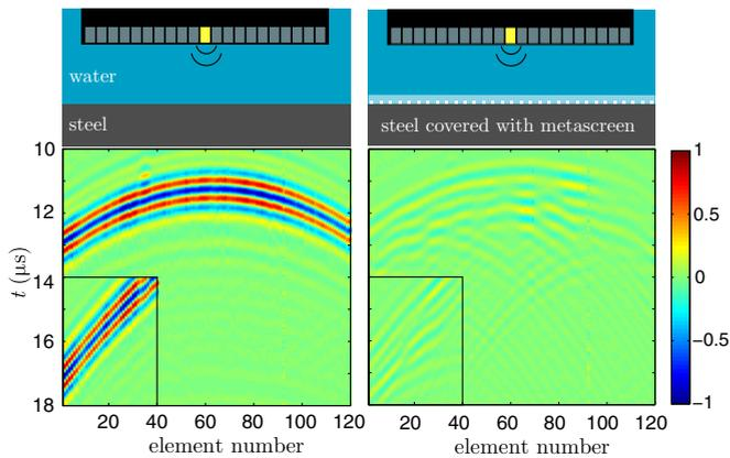
FIG. 4. (Color online) Pressure wave measured on each element of an array of transducers when a 2 MHz signal sent by an element in the middle is reflected either on the bare steel block (left) or on the same block covered with the optimized bubble metascreen (right). All the amplitudes are normalized by the maximum amplitude recorded in the bare block case. In the insets, the reflection of a tilted wave is recorded by emitting with the last element on the right.
