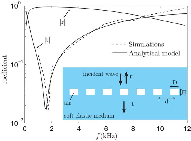
FIG. 1. (Color online) Comparison between Eq. (1b) and simulation data extracted from Fig. 16 in Ref. [20], for the transmission coefficient through a layer of air cylinders ( $H = 2$  cm,  $D = 1.5$  cm) on a square lattice ( $d = 5$  cm) in silicone.
