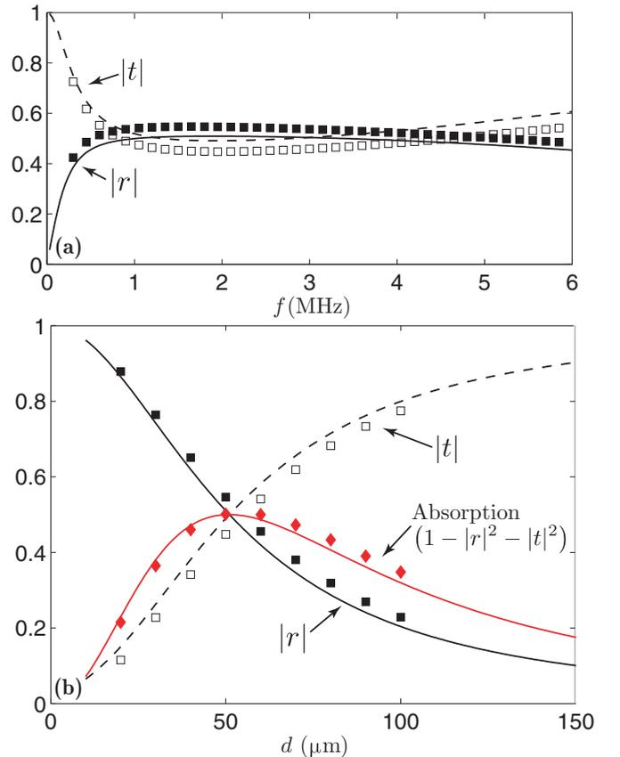
FIG. 2. (Color online) (a) Transmission and reflection predicted by the model (lines) and finite element simulations (symbols) for  $\eta = \eta^*$ . (b)  $|t|$ ,  $|r|$ , and absorption ( $A = 1 - |r|^2 - |t|^2$ ) at 2 MHz as a function of bubble spacing  $d$ .
