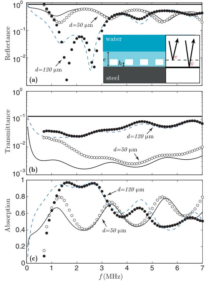
FIG. 3. (Color online) Experimental measurements (symbols) of the (a) reflectance, (b) transmittance, and (c) absorption for two different metascreens on a steel block. The solid thick horizontal lines are the values for the bare steel block. The solid and dashed lines show the prediction by the analytical model.
