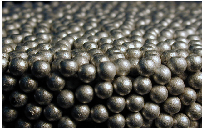
FIG. S1. Photograph of one of the samples. Note the small “necks” connecting the beads, whose spherical shape is preserved. The lightly polished top surface is also visible.
