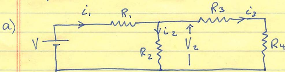
$$R_{\text{eff}} = R_1 + R_{\parallel} = R_1 + R_2 \parallel (R_3 + R_4) = R_1 + \frac{R_2(R_3 + R_4)}{R_2 + R_3 + R_4}$$
