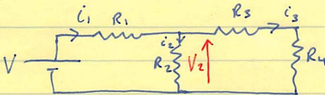
The voltage across  $R_2$  is  $V_2 = i_1 R_{11} = \frac{V}{R_{eff}} \left( \frac{R_2(R_3+R_4)}{R_2+R_3+R_4} \right)$
