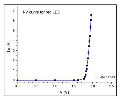
i) Use these data to estimate the resistance of the diode when it is conducting current.
