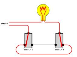
i) Denote the switches as S1 and S2, and assume they are set as indicated initially, with S1 off and S2 on, and the light is on.
