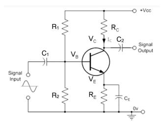
The suggested resistors are only approximate, so your operating point may not be as calculated in the prelab exercise. Use a DMM to check that the potential difference  $V_{CE}$  is close to 9 V. If it is not within  $\frac{1}{2}$  volt or so, you can vary  $R_1$  or  $R_2$ . Increasing  $R_2$  will increase the base current and reduce  $V_{CE}$ . Increasing  $R_1$  will do the opposite.
