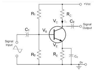
We will use:  $V_{CC} = 18$  V,  $R_I = 33$  k $\Omega$ ,  $R_2 = 2.2$  k $\Omega$ ,  $R_C = 3.3$  k $\Omega$ ,  $R_E = 220$   $\Omega$ ,  $C_I = C_2 = 0.47$   $\mu$ F,  $C_E = 10$   $\mu$ F.
