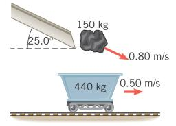
The coal is flying freely through the air and so  $v_x$  of the coal is constant while it is in the air.
