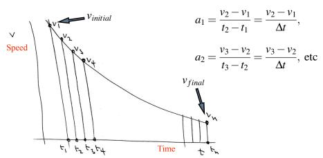
Work out the acceleration at each point, make all the time intervals equal:
