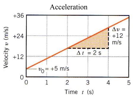
Acceleration =  $(12 \text{ m/s})/(2 \text{ s}) = 6 \text{ m/s}^2$
