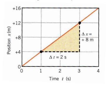
Average speed =  $\Delta x/\Delta t = (8 \text{ m})/(2 \text{ s}) = 4 \text{ m/s}$
