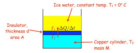
The rate of heat flow through the insulator is:  $\ \frac{\Delta Q}{\Delta t} = \frac{kA(T_2-T_1)}{d}$
