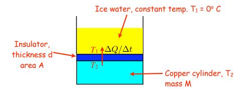
Heat flows from the copper cylinder, through the insulator to the ice water, which is kept at  $T_1$  = 0° C by the ice.
