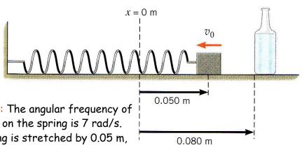
10.34/76: The angular frequency of the mass on the spring is 7 rad/s. The spring is stretched by 0.05 m, as shown, and the block is thrown to the left.
