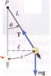
10.-/42: A pendulum clock acts as a simple pendulum of length 1 m. It keeps accurate time at a location where the acceleration due to gravity is  $9.83 \text{ m/s}^2$ . What must be the length of the pendulum to keep accurate time if the local acceleration due to gravity is  $9.78 \text{ m/s}^2$ ?
