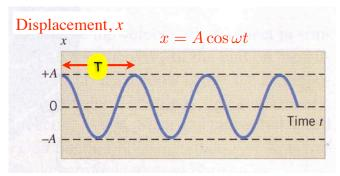
· SHM results when the restoring force is proportional to displacement:
