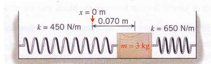
10.22: A 3 kg block is placed between two horizontal springs. The springs are neither strained nor compressed when the block is at x = 0. The block is displaced to x = 0.07 m and is released.
