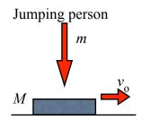
As the momentum of the person is downward, not sideways, the horizontal momentum of the boat is unchanged.
