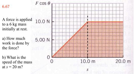
a) Work done = area under the force-displacement curve
