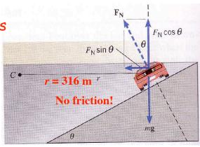
If  $\theta$  = 31° and r = 316 m, and there is no friction, what is the best speed to drive around the banked curve?
