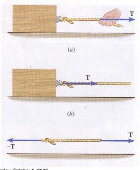
Tension - the force within a rope or cable that is used to pull an object.
