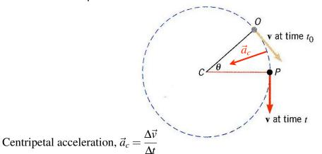
Work out the change in velocity in a short time interval...
