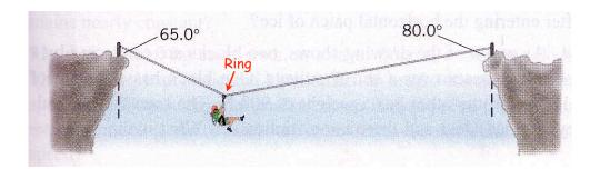
4.102/58: The mountaineer weighs 535 N. What are the tensions in the two sections of the cable?
