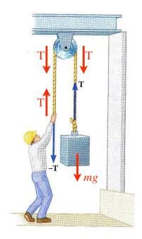
4.48/46: In the left hand diagram, the tension in the rope is 92 N. What is the tension in the right hand diagram?
