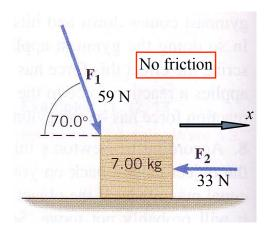
4.11: What is the acceleration of the block in the horizontal direction?
