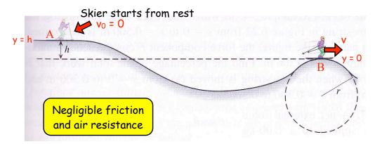
6.42: What must be the height h if the skier just loses contact with the snow at the crest of the second hill at B?
