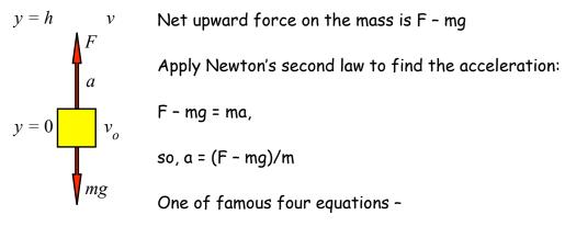
Net upward force on the mass is F - mg
