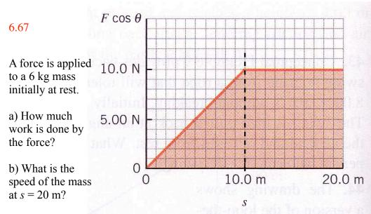
a) Work done = area under the force-displacement curve
