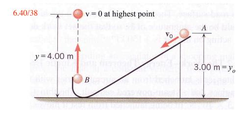
Find the speed of the particle at A  $(v_o)$ . There is no friction.
