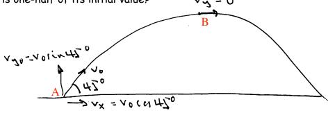
At any point:  $v = \sqrt{v_x^2 + v_y^2}$ , and  $v_x = v_0 \cos 45^\circ = v_0 / \sqrt{2}$
