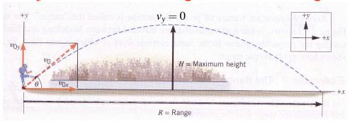
The projectile travels the horizontal distance R in the same time that is travels up to height H and back down to the initial height.
