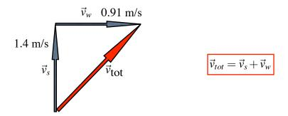
3.47/51: A swimmer swims directly across a river that is 2.8 km wide. He can swim at 1.4 m/s in still water ( $v_s$ ), i.e. at 1.4 m/s relative to the water. The river flows at 0.91 m/s ( $v_w$ ), i.e. at 0.91 m/s relative to the riverbank.
