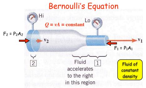
The fluid speeds up when it gets to the constriction. What is the force that causes this acceleration?
