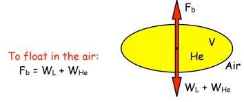
The buoyant force is,  $F_b$  = weight of air displaced by balloon =  $V \rho_{gir} g$  = 5400 × 1.2g = 63,500 N
