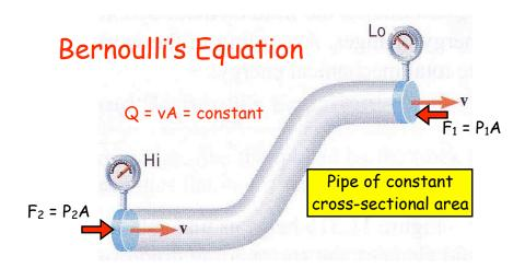
The fluid flows up hill at constant speed through a pipe of constant area. Where does the force come from to push the fluid up the hill at constant speed?
