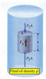
Buoyancy force =  $\rho$  Vg = weight of fluid displaced by the object
