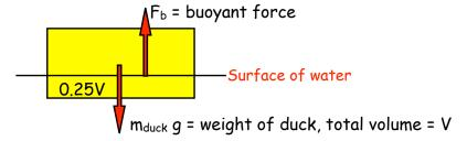
The duck floats, so the weight of the duck is equal to the weight of water with 25% of the volume of the duck.
