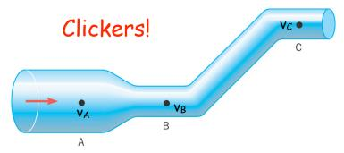
Fluid is flowing from left to right through the pipe. Points A and B are at the same height, but the cross-sectional areas of the pipe differ. Points B and C are at different heights, but the cross-sectional areas are the same.
