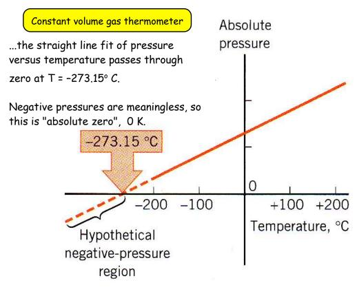
12.7: A constant-volume thermometer has a pressure of 5000 Pa when the gas temperature is  $0^{\circ}$  C. What is the temperature when the pressure is 2000 Pa?
