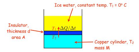
Heat flows from the copper cylinder, through the insulator to the ice water, which is kept at  $T_1 = 0^{\circ} C$  by the ice.
