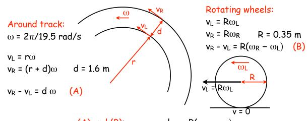
(A) and (B):  $v_R - v_L = d \omega = R(\omega_R - \omega_L)$
