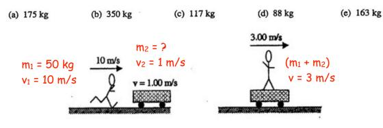
Conservation of momentum:  $m_1v_1 + m_2v_2 = (m_1 + m_2)v$ Solve for m<sub>2</sub>:  $m_2 = \frac{m_1(v_1 - v)}{v - v_2} = \frac{50(10 - 3)}{3 - 1} = 175 \text{ kg}$
