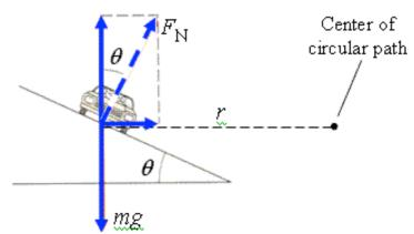
5.21/18: A car travels at 28 m/s around a curve of radius 150 m. A mass is suspended from a string from inside the roof.
