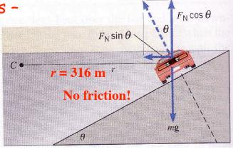
5.26/20: Two banked curves have the same radius. Curve A is banked at  $13^{\circ}$ , curve B at  $19^{\circ}$ . A car can travel around curve A without relying on friction at a speed of 18 m/s. At what speed can this car travel around curve B without relying on friction?
